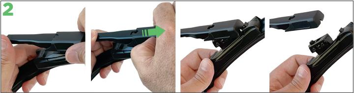
Hold the arm in position then slide the plastic cap forward into the unlock position to release the blade from the arm (you may need to press locking tabs).
