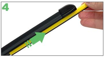
Remove the protective sleeve from the Ezywiper blade then place the arm back on the windscreen.
