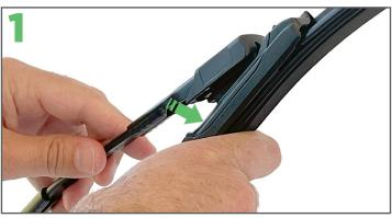
To remove the current wiper, rotate the blade away from the arm as far as it will go.
