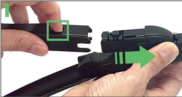
1 To remove the current wiper blade push the button down and slide the blade away from the arm.
