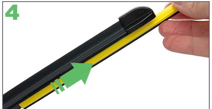
4 Remove the protective sleeve from the Ezywiper blade then place the arm back on the windscreen.
