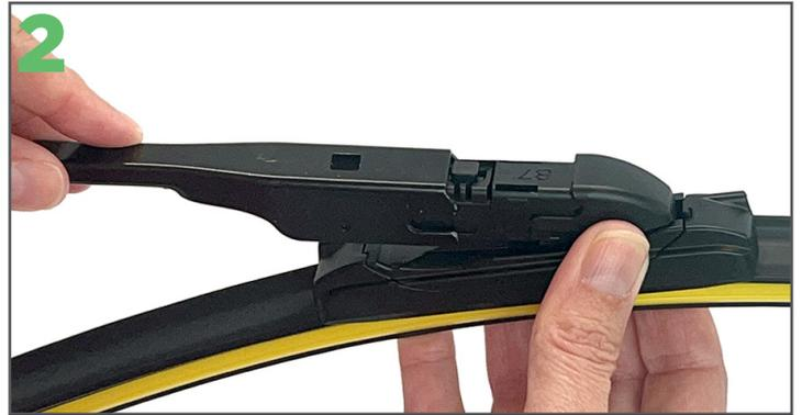
2 Next, remove the new Ezywiper blade from its packaging. To fit the Ezywiper blade, line the wiper blade up with the arm.
