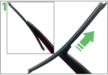
1. Lift the wiper blade off the rear screen (inset) then gently tilt the blade until it is at 90° to the arm.
