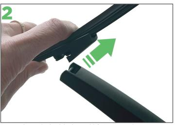
2. Gently rock the blade and lift it upwards so it disengages from the arm.
