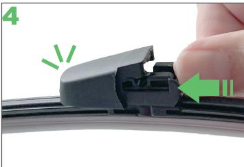
3. Retrieve the new wiper blade and position it so you 4. Slide the adaptor in the direction of the arrow on the mount until the adaptor clicks into place.
