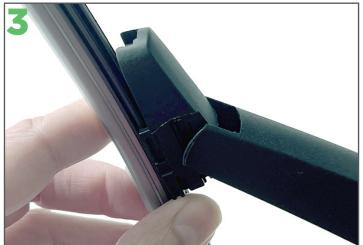
3. To fit your new Ezywiper blade, hold it at 45° to the 4. Gently push the blade onto the arm until it locks arm and gently place it position on the arm.
