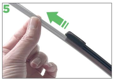
5. Don't forget to remove the protective sleeve from the new blade before placing the arm back on the rear screen.
